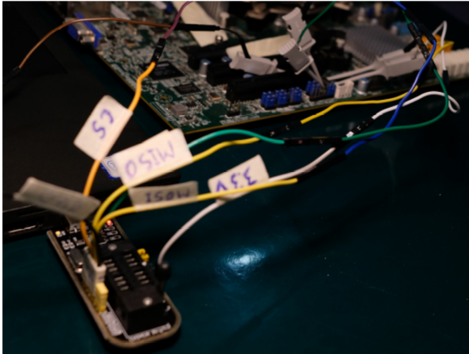
Fig.11: test grabbers connected to the "CH341A" programmer inserted into the researcher's laptop
